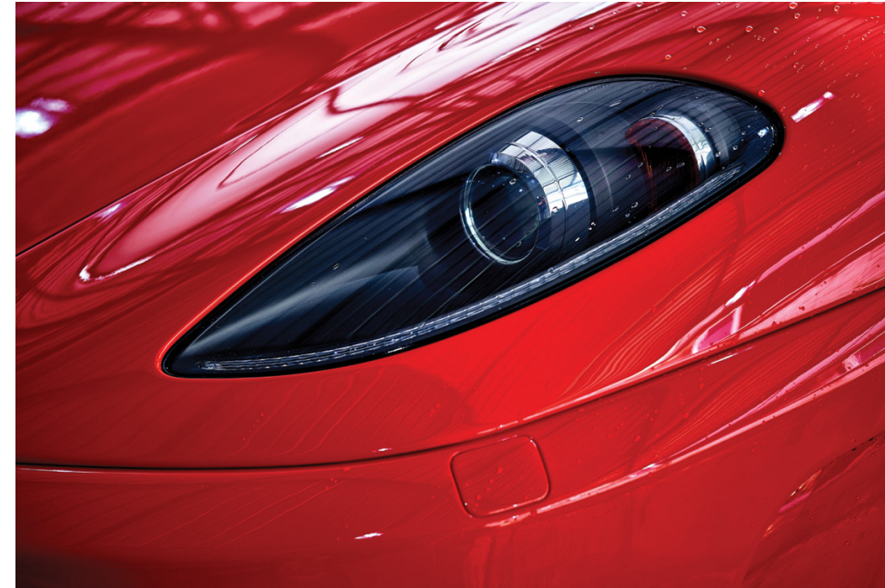
Figure 04. UV-cured coatings protect plastics used in the production of automotive headlights from abrasion, wear and impact damage.
